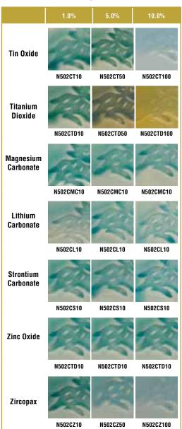
Opacifiers were added to glaze base N502 in increments. The chart above shows which materials were added for this purpose, and the percentages tested. All glazes in this test batch also had 1% copper carbonate added to increase the visual effect of the chemicals on the glaze.
