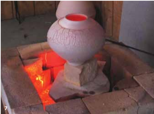
7 After the kiln reaches 1450°F, remove the pot with raku tongs and place it in the metal can reduction chamber.
