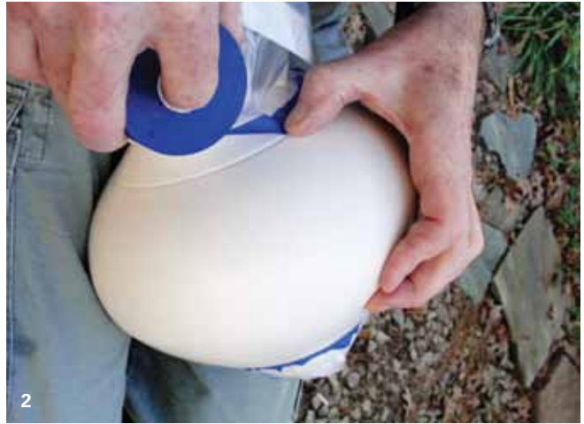
2 Mask off the areas you want to remain black using house painter's tape.
