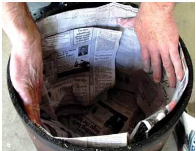
6 While the pot is in the kiln, line a steel can that is slightly larger than the pot with several sheets of newspaper.
